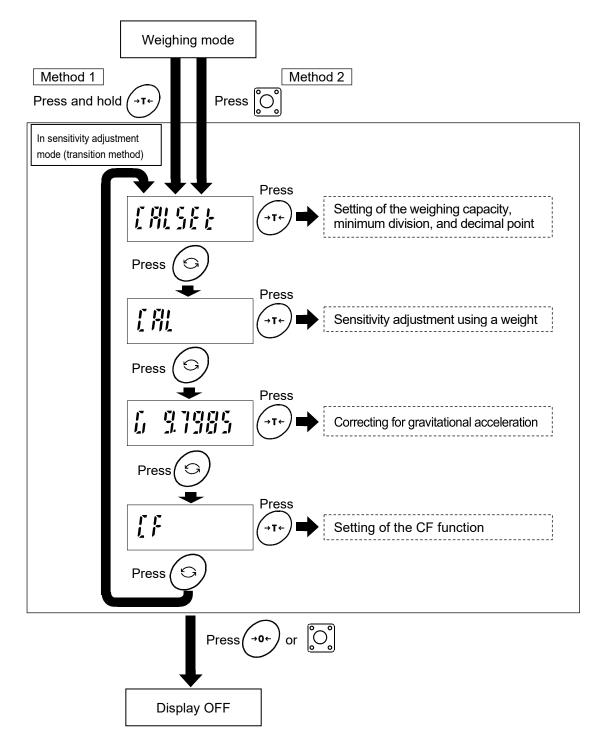
Note: Use the MODE key to select the item to execute, and then execute with the TARE key. Note: To end sensitivity adjustment mode, press the ZERO key or CAL switch. The display turns off. (You can also turn it off using the ON/OFF switches.)
