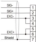
(A) 6-wire configuration connection to load cell (recommended)
